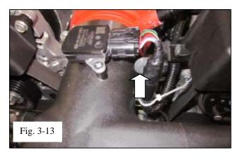
(m) Plug in the MAF sensor wire harness; secure the MAF sensor wire harness to the TRD Air Box with supplied zip tie. (Fig. 3-13)
