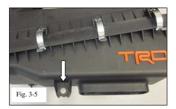
(e) Transfer two of the grommets from the OEM air box to the TRD Air Box. (Fig. 3-5)
