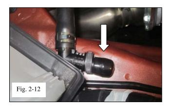
(l) Cap off the fitting on the frame rail with the supplied cap plug. (Fig. 2-12)
