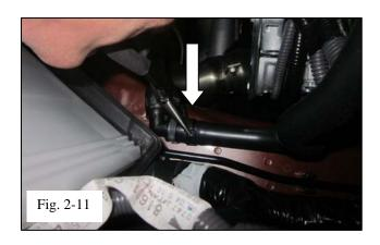
(k) Detach the Sound Generator tube from the fitting on the frame rail by squeezing the spring clamp. (Fig. 2-11)(1) Remove the complete Sound
