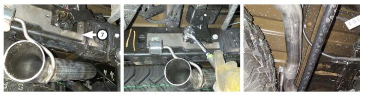
Place clamp (8) and rear hanger mount (removed step 3) onto left exit pipe (5) then connect it to y-pipe left outlet. Re-install rear hanger mount then tighten clamp just enough to allow for later adjustment.
