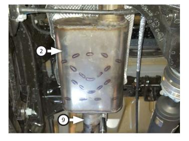
Route y-pipe (3) over rear axle and connect it to muffler, simultaneously inserting wire hanger into isolator. Tighten clamp just enough to allow for later adjustment.
