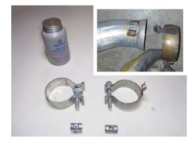
www.flowmastermufflers.com Technical Support (866) 464-6553  Place factory ball clamp (removed step 5) onto inlet pipe (1) then connect it to catalytic converter. Insert wire hanger in isolator and tighten clamp enough to allow for adjustment.
