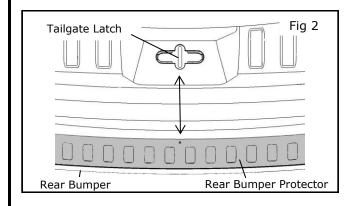
3) Dry fit the bumper protector on the vehicle by aligning the bumper protector centering arrow with the tailgate latch. (Fig 2)
