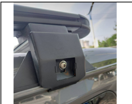
10. Put the frame of the assembled bracket on the roof of the vehicle, adjust the bracket to the proper position on the roof, and fix it with screws.
