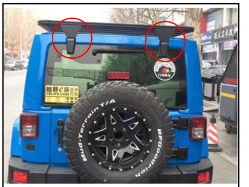
12. Unfasten the plastic cover at the rear of the car, unscrew the screws, and place the brackets corresponding to the screw holes, then tighten the screws, and finally close the cover.
