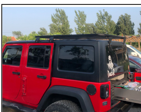
11. As shown in the figure, install the rear bracket, the bracket corresponds to the screw hole position, lock and fix.
