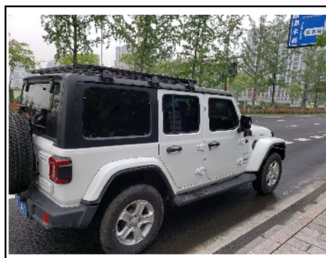
11. The flat roof basket is installed.
