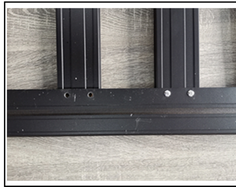
5. Install the bottom plate, match the bottom plate to the hole of the frame, and fix it with screws.
