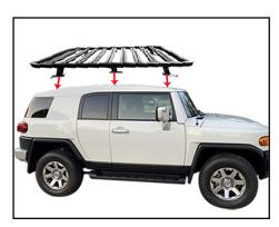
10. Align the bracket's holes with the car roof original holes, and lock it tightly.
