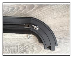
Install corners and connect the corners to the frame.
