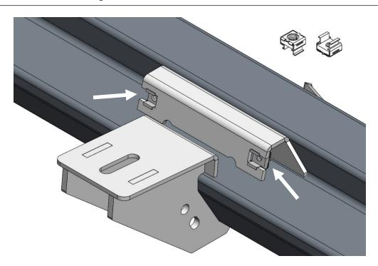
**Step. 3** Carefully raise step rail up to the pinch weld of the body and align brackets up with the factory mounting locations.
