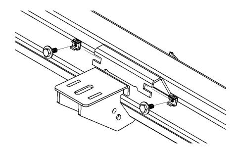
**Step. 7** After finial positioning, tighten all (x6) 5/16 "x ¾" hex bolts no more than 6 ft/lbs. torque.
