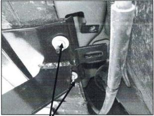
10mm x 30mm Hex Head Bolts 10mm Flat Washers 10mm Lock Washers 10mm Hex Nuts
