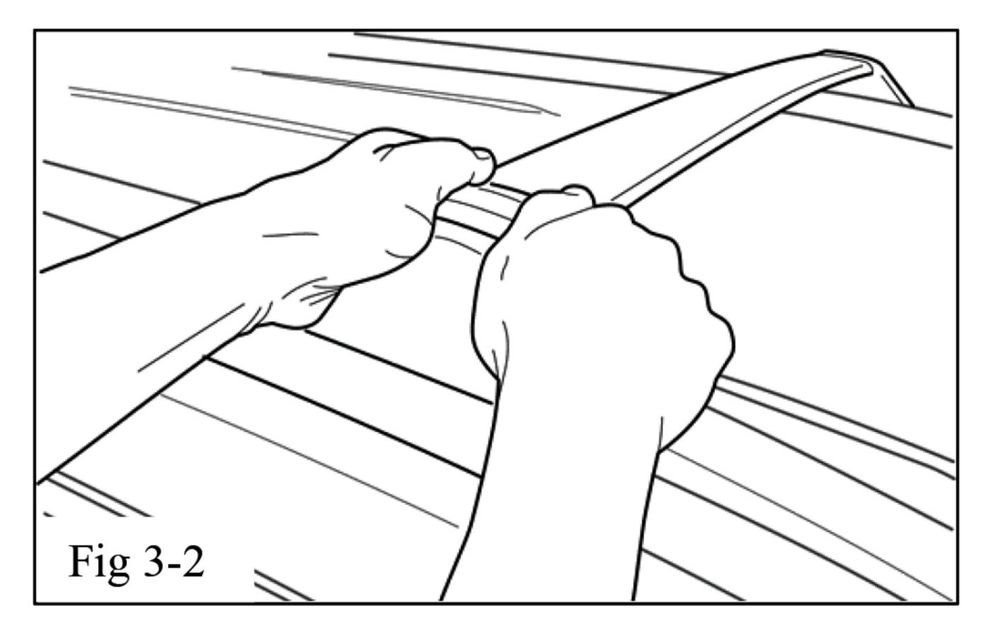
(b) Rotate the top of the cover toward the stanchion and use both hands to firmly press to snap the top and side tabs into place (Fig. 3-2).
