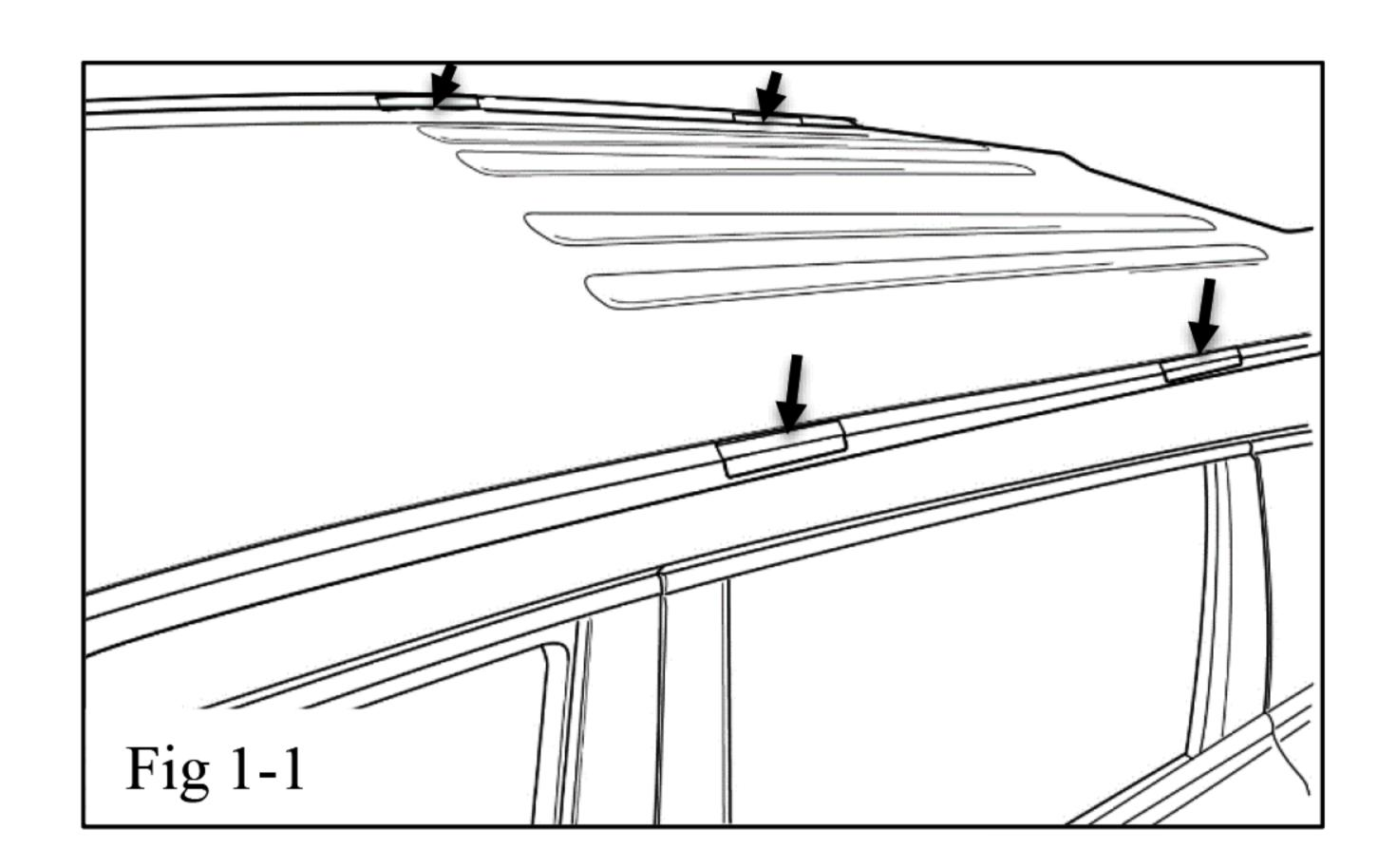
(a) Locate 4 covers on side rails on roof of vehicle (Fig. 1-1).
