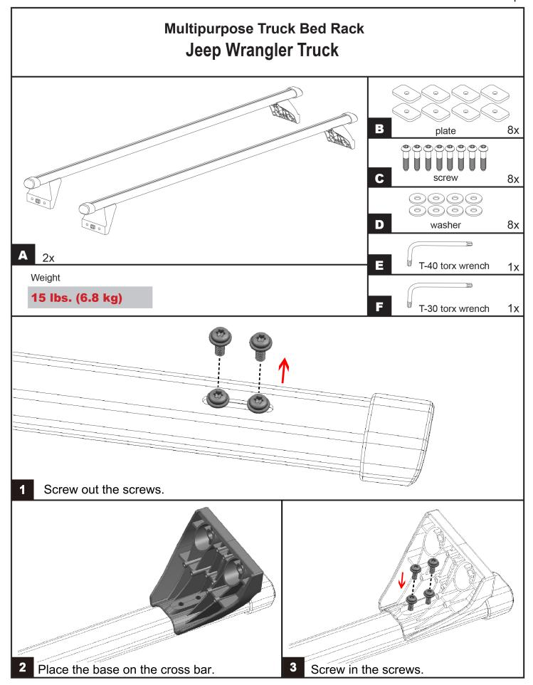
4) Loosely attach the screws, washers and nut plates to each of the 4 towers with the T-40 torx wrench.
