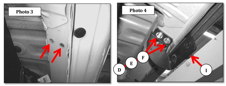
**Step-4** Attach the passenger side center bracket to the body panel using (2) M8 hex bolts, (2) 5/16" lock washers and (2) 5/16" flat washers. Leave the nut and bolts loose for final adjustment, (Photo 4).
