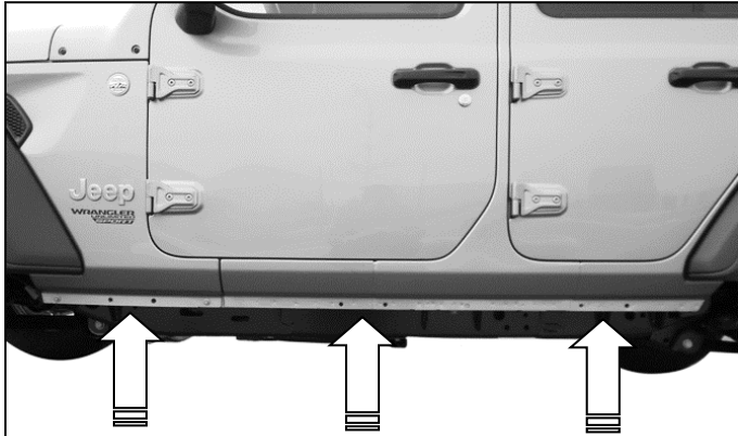
(Fig 1) Locate the (3) factory pair of holes along the pinch weld (Driver/left side pictured)
