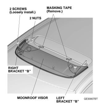
12. Install the brackets agianst the body as shown. NOTE: Read the IMPORTANT INFORMATION label to avoid wind noise.
