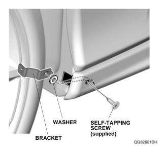
16. Secure the left rear splash guard with two washer-self-tapping screws in the order shown below. NOTE: Make sure there is no gap between the left rear splash guard and the bumper. If there is a gap, loosen the washer-self-tapping screws, hold the splash guard against the bumper, and retighten the screws.
