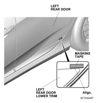
11. Using an alcohol swab, thoroughly clean the area where the left rear door lower trim will attach.
