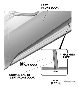
2. Using an alcohol swab, thoroughly clean the area where the left front door lower trim will attach.
