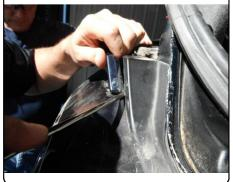
6. Remove (1) fastener from underneath each piece of trim removed in STEP 5.
