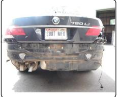
9. Place hitch into position over threaded studs and place bumper beam over hitch. Clamp hitch between vehicle trunk pan and bumper beam using the nuts removed in STEP 8. Torque all M10 hardware to 48 ft-lbs.
