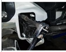
5. Raise hitch into position aligned with vehicle studs and secure using supplied M12 hardware.
