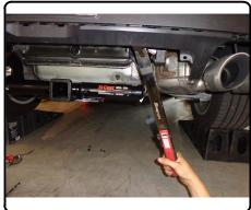
9. Porsche models: Raise rear fascia up into position and mark around side plate interference where fascia needs to be trimmed. Approx. 1/2" by 1" each side. Trim area with either a cut-off wheel or shears. After fit is confirmed, clip fascia back into position by following Steps 1-2 in reverse.
