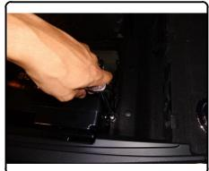
6. Porsche models (2009-2016): With trunk components cleared for drilling, mark drill holes through hitch mounting holes on underside of pan. Drill 1/2" holes for mounting hardware. NOTE: 2017 models do not require drilling.
