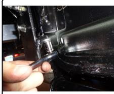
5. **Porsche models**: The trunk pan mounting holes must be drilled. Open trunk to clear vehicle components for drilling. Remove floor panels and spare tire, set aside. Disconnect battery terminals with a 10mm socket, remove audio module by removing (2) T-27 Torx screws. Disconnect battery strap using a 13mm socket and extension.
