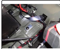
8. In sequence, torque 1/2" hardware to 110 lb-ft, 8mm bolts to 23 lb-ft, and 3/8" u-bolts to 45 lb-ft. Reinstall lower bumper fascia by following Steps 1-2 in reverse.
