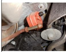
2. Remove rear heat shield at vehicle fascia by removing 4 hex bolts and 8 Torx bolts. Heat shield may either be trimmed and reinstalled or permanently removed.
