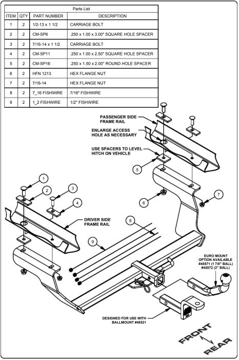
1) Remove the (4) plugs in the frame rails and return to vehicle owner (leave center plugs in).
