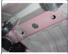
2) Fishwire 7/16" carriage bolts and CM-SP11 spacers into position first and reverse fishwire 1/2" carriage bolts and CM-SP6 spacers into position afterward. (enlarge access hole as necessary)
