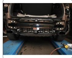
10. Torque all 12M fasteners to 82 ft-lbs and reinstall all components removed in steps 1-7
