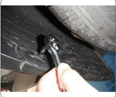
3. Remove fastener which holds wheel well trim to fascia. Carefully pop off wheel well trim. **Note:** Only the rear half of the trim needs to be removed.
