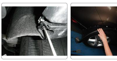
4. Remove (4) torx head fasteners from under wheel well trim.
