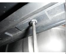
Remove mud flap from behind each rear tire by unfastening (5) torx head screws from each. Note: Underside fasteners have a nut attached.
