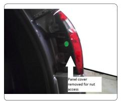
Remove (2) torx head fasteners and (1) push fastener from each side. These are now accessible due to tail light removal. Note: Use a small punch or equivalent to push the center of push fastener down then pry up.
