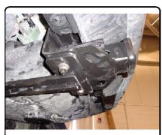
15. Secure the (2) center fascia tabs by pushing the nylon retainer clips into the holes in hitch tube.
