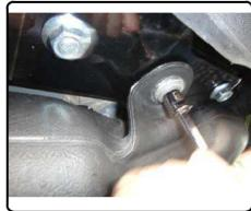
12. Raise and secure the exhaust lowered in Step (3). BlueTEC vehicles only, reinstall DEF tank shield removed in Step (1).
