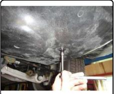
13. Raise mounting strap (B) into position and loosely secure to hitch 1/2-13 x 1" carriage bolts and 1/2-13 hex flange nuts. Raise nut plate (C) into position and secure mounting strap to the cross member using 1/2-13 x 3" hex bolts and 1/2" conical toothed washers.
