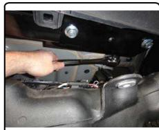
11. BlueTEC vehicles only, raise DEF tank and secure the mounting strap using hardware removed in Step (5). Secure DEF tank mounting tab using M8-1.25 x 40mm hex bolt and 3/8" conical toothed washer. Secure driver side using M8-1.25 x 30mm hex bolt and 3/8" conical toothed washer. Torque M8 hardware to 23 ft-lbs.
