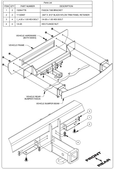
1. On the fascia tab bracket, locate and remove (2) screws from rear fascia and (1) nut located on top of bracket using 10mm socket. Remove bracket and return to owner.
