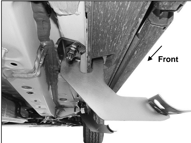
(Fig 17) Passenger/Right Center Bracket installed
