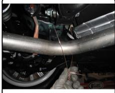
2) Remove the heat shield by removing the 4 small screws with a 10mm socket. Cut a hole in the heat shield as shown in the diagram to left.
