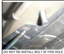
5) Raise hitch into position. **Note:** The heat shield will be sandwiched between the hitch and vehicle frame rails.
