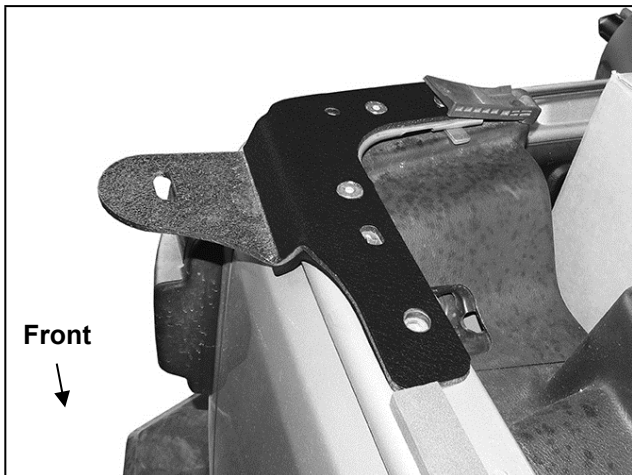
(Fig 14) Passenger/right Mounting Bracket installed
