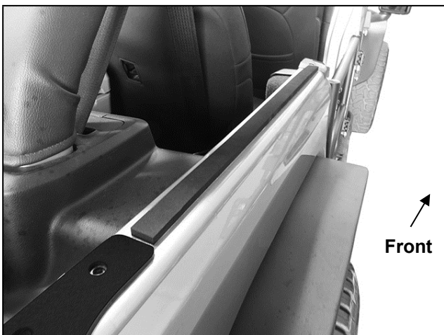
(Fig 16) Install Foam Seal in original location
