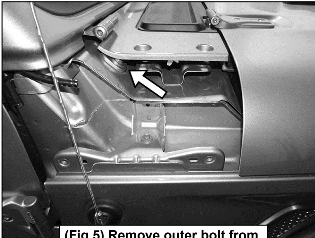
(Fig 5) Remove outer bolt from windshield hinge (arrow)
