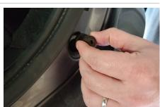
Gently pull enough of the wheel well trim out to remove the rear fascia on both sides of the vehicle. Gently remove the rear bumper fascia by pressing the three clips on the rear bumper fascia on each side, gently pulling the rear bumper fascia off the vehicle, and unplugging one or two connectors from fascia.
