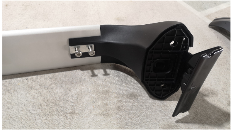
4. As shown in the picture, put in the spacers, and then tighten the screws
