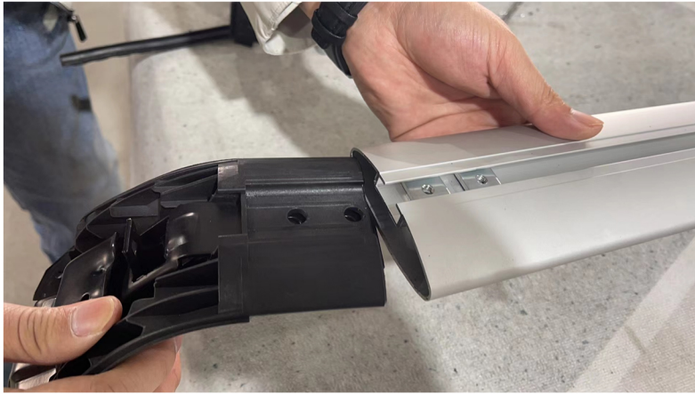
3. As shown in the picture, slide in the box screws, and then install the lower bottom cover
