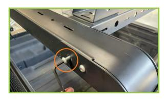
3) Using an allen wrench, remove the existing button head screw from each front leg. Only remove the inside screw on each side as shown above. Once removed mount the Head Panel and secure each of these locations with the 3/8" -  $16 \times 1.0$ " Button Head Screw and a Flange Nut. Lightly tighten for now so that you have room for adjustments.
