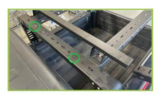
4) Using (2) 3/8" -  $16 \times 3/4$ " Button Head Screws and (2) Flange Nuts secure the top flanges from the Head Panel to the transverse crossbar in the locations as circled above. Lightly tighten for now so that you have room for adjustments.
