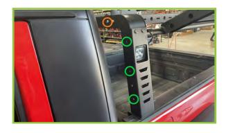
5) Secure the Head Panel to the front legs using (3) 3/8" - 16 x 3/4" Button Head Screws and (3) Flange Nuts for each side.
