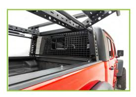
6) Tighten all hardware once each screw has been threaded to a flange nut. This completes the installation guide for Z384031.
