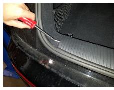
On the inside of the trunk locate (2) rubber plugs,
