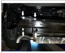
8. Raise hitch into position along with the bumper beam and bumper beam bracket and secure with hardware removed from step 7. Torque M10 hardware to 45 ft-lbs.
