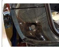
4. Remove trunk floor and use plastic pry tool to remove trunk edge trim starting from the side.
