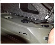
6. Remove access panel on either side of trunk and locate (2) nuts, (1) on either side, and remove using a 10mm socket.
