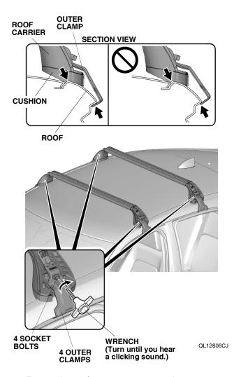
6. Ensure the roof carriers are secured.
