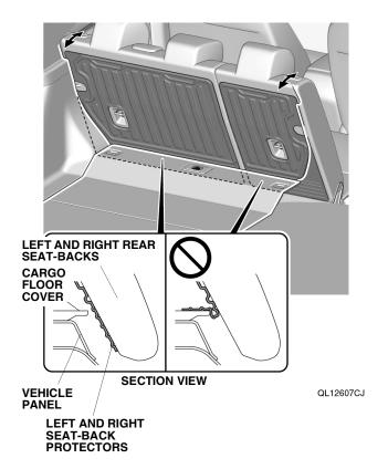
7. Check that all parts are installed properly.
