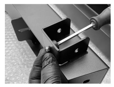
6. Install the rubber stop to each of the (4) legs. Use (1)  $6-32 \times 3/4$ " machine screw and (1) 6-32 nylon lock nut for each stop.
