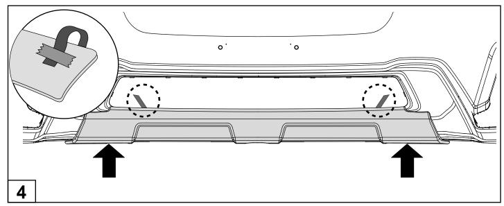
Install Front Bumper Under Guard in position of best fit ensuring that folded tape liners remains outside.
