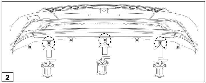
Identify the (3) locations of the factory retainers in underside of bumper and remove with either Philips head screwdriver or plastic pry bar. Discard the 3 retainers.
