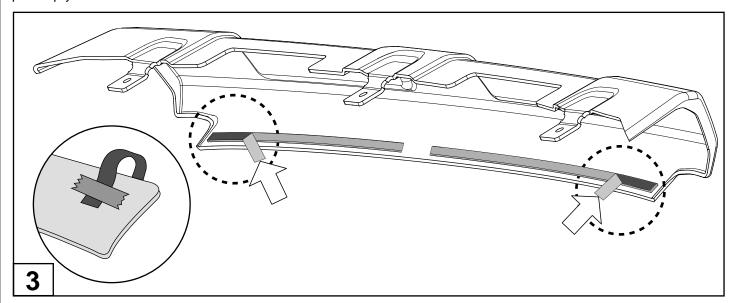
Peel back approx. 50mm / 2" of tape liner at each end of the part and fold at 45 degrees to part. Tape peeled back section of tape liner to outside surface of the bumper under guard using masking tape.
