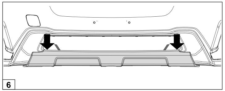
Apply moderate forward pressure towards bumper for product best fit, then apply pressure to the ends of the Front Bumper Under Guard where the double sided tape liner has been removed, (as shown).
