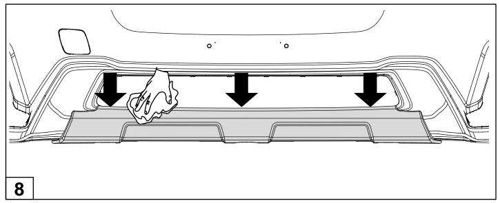
With a clean, dry microfiber towel, apply pressure to taped surface of Front Bumper Under Guard, (as shown) going from side to side approx. 5 times to ensure proper tape adhesion is achieved.
