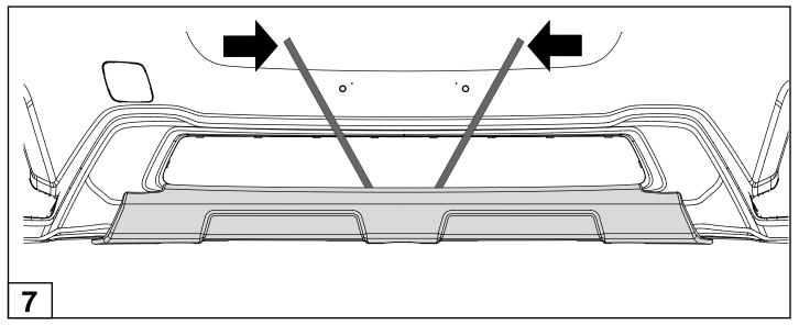
While applying moderate forward pressure towards bumper, pull exposed tape liners towards opposite end of Front Bumper Under Guard, one side at a time (as shown).
