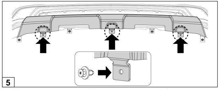
Install (3) provided replacement retainer plugs in (3) available holes in Front Bumper Under Guard.
