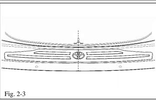
(c) Before installing the rear bumper protector, ensure the central arrow is aligned with the center of the vehicle or lift gate striker (Fig. 2-3).
