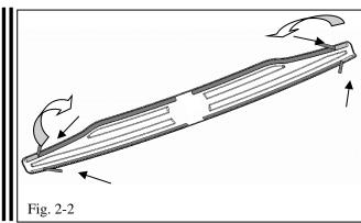
(b) Ensure all the tabs are folded so they can be accessed from the top once the protector is seated on the rear bumper (Fig. 2-2).
