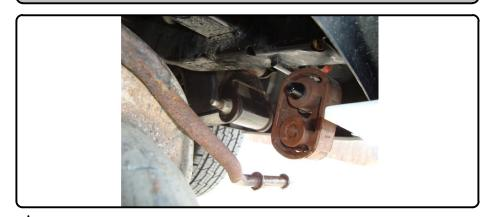
2. Locate 2 holes in vehicle crossmember, which correspond to slots in hitch side arms, and enlarge with 1/2" drill bit (See View A).
