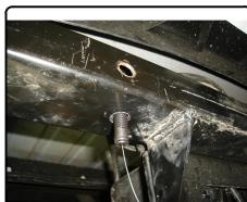
4. Raise hitch into position and install 1/2-13 X 4" lg. carriage bolts, blocks and 1/2-13 hex flange nuts loosely, as shown.
