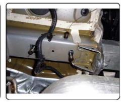
4. Raise hitch up from in front of the exhaust and into position, using care not to push hardware back inside frame. Be sure to loosely secure hitch with the mounting hardware to align all holes before tightening. Note: S eam foam may need to be trimmed for proper
