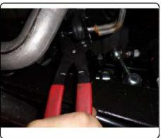
2.) Fishwire the carriage bolts and small square hole spacers through the space between the bumper beam and the end of the frame rail for both sides.
