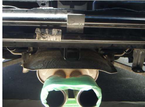
Photo 8: Hitch in position.
