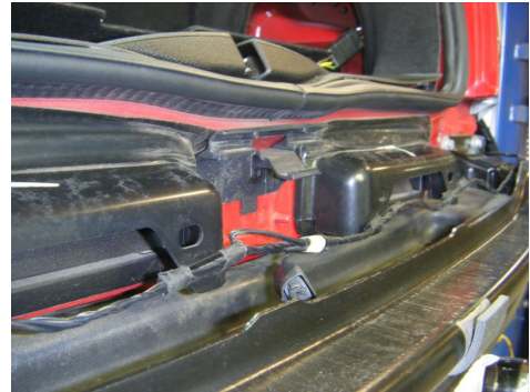
Photo 12: Center alignment feature.
