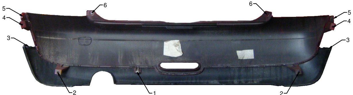
Photo 2: Fastener locations as viewed from inside of the bumper cover. (These fastener locations are present on all models.)
