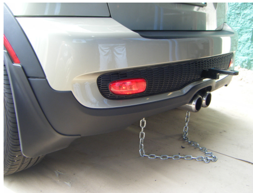
Photo 13: Hitch shown installed with safety chains
