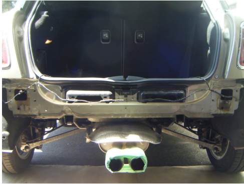
Photo 7: Bumper beam removed.
