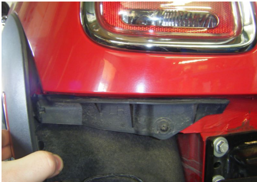
Photo 11: Side alignment feature.
