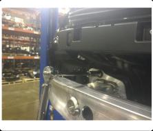
11. Trim bumper fascia as shown in the trim diagram using aviation shears.
