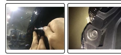
Inside the trunk along the plastic liner guard use plastic pry bar to remove (2) caps, (1) on each side, to access and remove (2) T45 bolts, (1) on each side using T45 Torxbit Socket.
