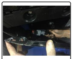
Remove the bumper beam by removing (8) M10 nuts using 15mm socket, (4 on each side). Set aside bumper beam for reinstallation in step 12.
