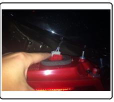
7. Gently remove rear bumper fascia by releasing the press-in tabs along top portion of bumper fascia. Unclip motion sensor harness on the driver side of vehicle. Set aside for reinstallation in step 12.
