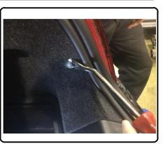
To remove taillights, locate and remove (8) M5 nuts using 8mm socket, (4) on each side. Unclip electrical harness and gently remove taillignht, set aside for reinstallation in step 12.
