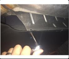
3. Pull back wheel well cover to remove (2) M4 screws using 7mm socket (1) on each side.
