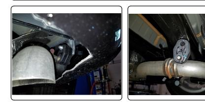
Locate and remove (2) plastic nuts with a 10mm socket. Remove heat shield and mark out a 5" x 13" section with masking tape. Use aviation shears to trim marked area. Reinstall with (1) nut using a 10mm socket.
