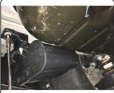
6. <u>On Hybrid models only:</u> enlarge holes on driver side frame rail using die grinder as shown in the Hole Enlargement Diagram
