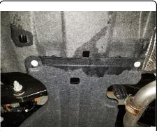
Locate and remove (3) screws from driver side wheel well with an 8mm socket. Remove underbody panel and mark out a 0.5" x 10" slot with masking tape. Use aviation shears to trim underbody panel. Set aside for later reinstallation.
