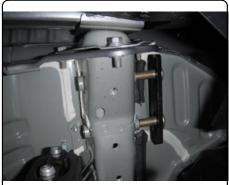
Raise hitch into position and slide the bolts through to support it. Loosely install the supplied hex flange nuts and the (2) hex bolts and conical washers as shown. Be sure teeth on washers are against the hitch mounting plate.
