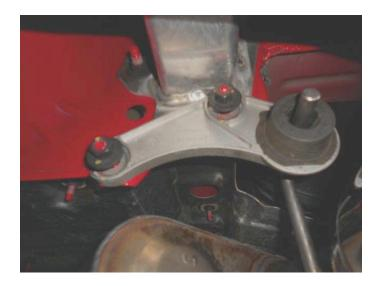
5. Carefully deburr factory pipes at cut ends. Remove hanger mounts at rear of vehicle from vehicle frame and transfer them from factory system to corresponding side on Flowmaster system.
