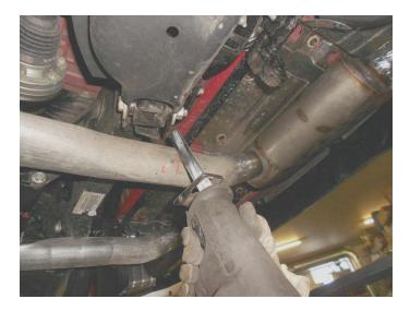
4. Remove hangers (x2) at front of muffler from isolators on vehicle. With help, slide system forward and out of rear hanger mounts. Lower system to floor with front hangers attached.
