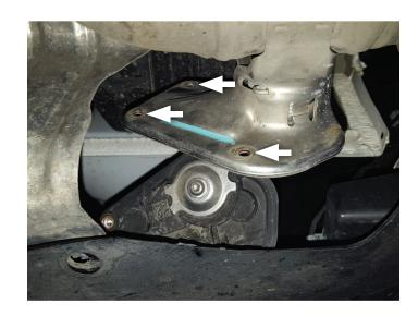
7. Remove screws (x2 ea.) from muffler/pipe hangers then dismount muffler wire hangers from their mounts in front of driver and passenger side muffler outlets.
