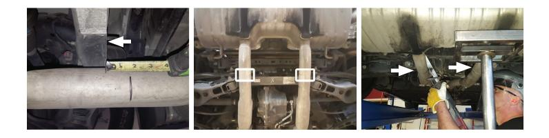
4. Dismount both front wire hangers, remove nuts (x4) and muffler/pipe hangers (x2) from muffler rear then disassemble and set aside muffler from vehicle. Retain nuts and muffler/pipe hangers for later use.
