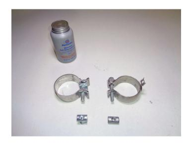
www.flowmastermufflers.com Technical Support (866) 464-6553  Place clamps (x2) (3) onto left (1) and right (2) mufflers then connect them to exhaust and insert wire hangers (x2) into isolators. Secure muffler ends with nuts and muffler/pipe hangers (removed step 4).
