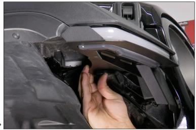
17. Attach the inner fender to the body of the Jeep using the same hardware (bolts and push rivets) you removed earlier.
