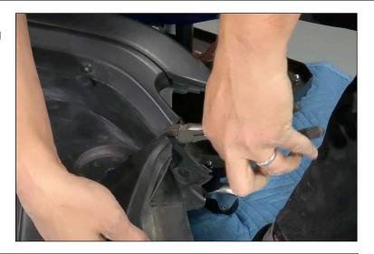
11. Each light is marked L (Passenger Side) and R (Drivers Side). Take the light and plug to the OE harness. Be sure the press the gray tab in after the harness is fully pushed in, this will lock it together. Lay the wire of the light in the fender braces. Take tie wraps and secure the wire to the braces.
