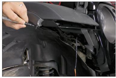
14. Install the bracket to fender brackets to the main bracket. The fender top side bracket mounts as shown in "A". Use M6 hardware to attach.
