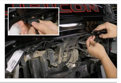
12. Reinstall all the fender clips to the fender. Then attach the fender back to the Jeep.
