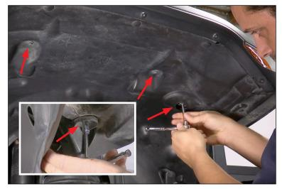
2. Use a pry tool to remove the push rivets holding the liner to the body of the Jeep.
