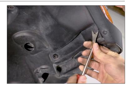
3. To remove the fender from the body start from either the bottom corner or front and pull away. The fender is attached with clips to the body, yanking the fender is the best method to release.
