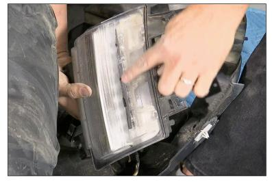
8. Remove the light harness from the fender. You'll have to pull back the liner to expose the retainers to pull from the fender. If you struggle pulling the retainers away either use the pry tool to remove or cut the retainers with snips.
