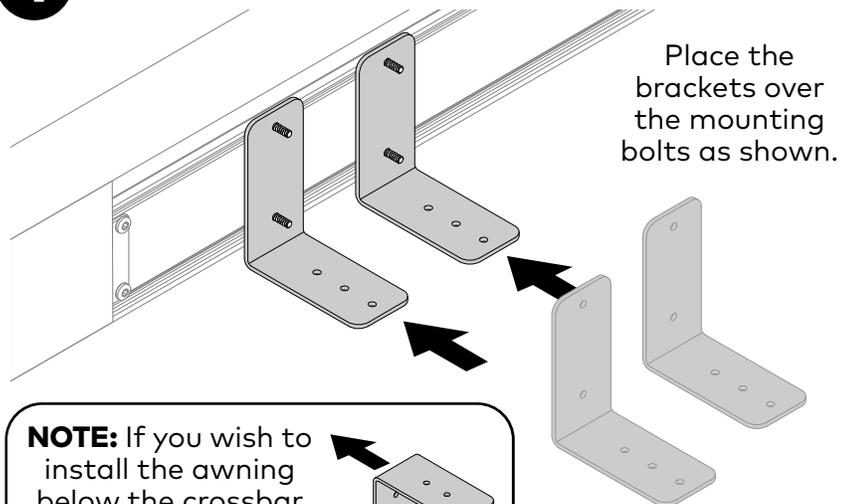
Place the brackets over the mounting bolts as shown.
