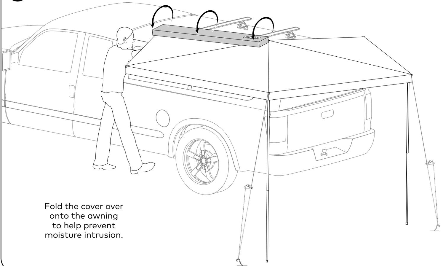
Fold the cover over onto the awning to help prevent moisture intrusion.
